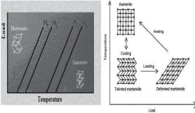
**Fig: 4.** The Dependency of Phase Change Temperature on Loading
