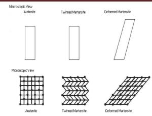
**Fig: 3.** Microscopic and Macroscopic Views of the Two Phases of Shape Memory Alloys
